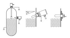
For flush mounting, the sensor can be built into influencing material up to its active surface without changing its characteristics. For non-flush mounting, a metal-free zone around the sensor must be allowed for. A free zone to the material opposite the sensor must be maintained for all sensors.
