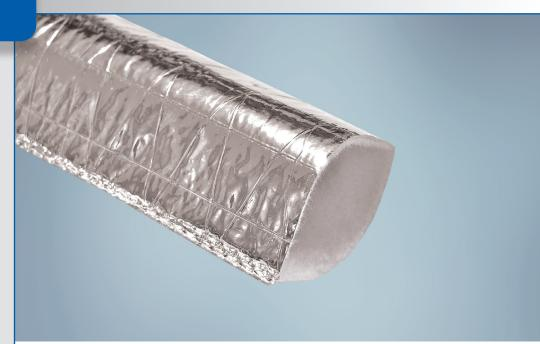
**ReflectSleeve® 1501** is reinforced, aluminized polyester sleeve designed to protect components in high temperature environments. The external surface is composed of a highly reflective aluminum foil, which provides radiant heat protection for internal components. The internal layer is composed of a polyester non-woven material, which provides added insulation efficiency. A layer of fiberglass scrim contributes to both product flexibility and durability.
