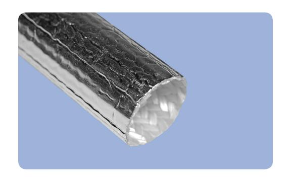
**ReflectSleeve**<sup>®</sup> **1451** is a one-piece fiberglass sleeve that is laminated to an aluminum foil. A special manufacturing process permits the sleeve to boast a virtually seamless and non fraying construction. This feature makes ReflectSleeve 1451 a low profile solution easily applied to the application it protects. The outer aluminum finish is highly reflective while the inner layer of the fiberglass greatly increases insulating efficiency.
