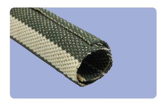
**ROUNDIT**<sup>®</sup> **2000 NX HT** is a self-wrapping sleeve manufactured from PEEK monofilaments and Nomex<sup>®</sup> multifilaments. It includes a water repellent treatment in order to prevent the absorption of condensation build-up caused by the extreme changes aircraft are subjected to. Designed for mechanical protection and maintenance of wire and cable bundles, its 100% covering ratio provides excellent cut-through and abrasion resistance.
