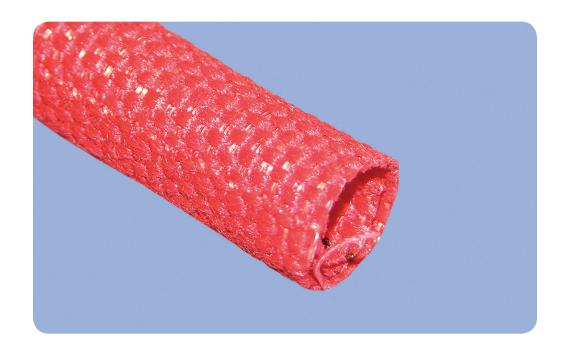
**ROUNDIT® 2000 NX** is a self-wrapping sleeve manufactured from PPS monofilaments and Nomex® with an oil and water repellent treatment, designed for mechanical protection and maintenance of wire and cable bundles. Its construction with 100% covering ratio provides excellent cut-through and abrasion resistance.
