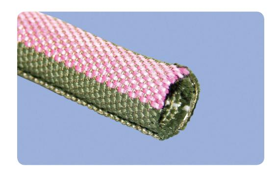
**ROUNDIT® 2000 NX Ptr** is a self-wrapping sleeve manufactured from PPS monofilaments and Nomex<sup>®</sup> multiflaments with an oil and water repellent treatment, designed for mechanical protection and maintenance of wire and cable bundles. This design allows for 100% coverage providing excellent cut-through and abrasion resistance.
