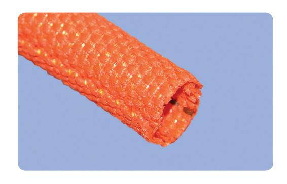
**ROUNDIT® 2000 NX** is a self-wrapping sleeve manufactured from PPS monofilaments and Nomex<sup>®</sup> with an oil and water repellent treatment, designed for mechanical protection and maintenance of wire and cable bundles. Its construction with 100% covering ratio provides excellent cut-through and abrasion resistance.
