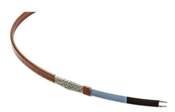
nVent RAYCHEM QTVR self-regulating trace heating cables are suitable for freeze protection of large pipes/vessels with high heat loss, and for process temperature maintenance applications without steam-cleaning requirements, up to 225 °F/110 °C. The fluoropolymer outer jacket (-CT) provides high chemical resistance against aggressive organics and corrosives.
