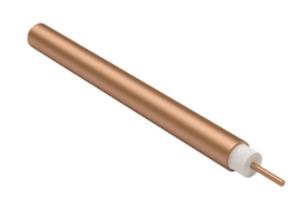
nVent RAYCHEM mineral insulated (MI) series resistance trace heating cables are used for low temperature maintenance applications such as long pipeline heating, condensation prevention and ramp heating. Copper sheath with continuous exposure temperatures to 392 °F/200 °C and typical power outputs to 20 W/ft (65 W/m). Approved for use in hazardous areas.
