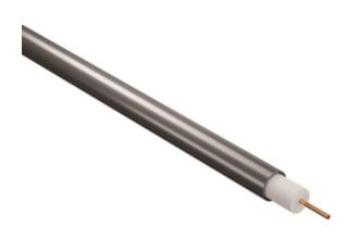
nVent RAYCHEM HSQ stainless steel (321) sheathed mineral insulated (MI) series resistance trace heating cables provide freeze protection and process temperature maintenance. They can be used for exposure temperatures up to 700 °C (joint dependent) and typical power outputs up to 150 W/m. 321 stainless steel sheath offers high corrosion resistance to a wide range of organic acids and alkalis. Approved for use in hazardous areas. Available 'fast track' as configured heating units.
