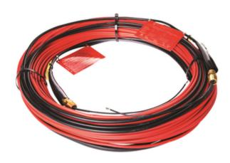
nVent RAYCHEM LSZH jacketed copper sheathed mineral insulated (MI) series resistance trace heating cables are used for low temperature maintenance applications including embedded heating in concrete or asphalt, roof de-icing, frost heave protection, exposed snow melting and interior pipe tracing. Continuous exposure temperatures to 194 °F/90 °C and typical power outputs to 35 W/ft (115 W/m depending on application.) Embedded and roof de-icing applications approved for use in hazardous areas.
