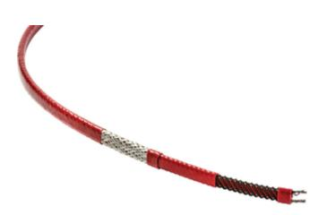
nVent RAYCHEM KTV self-regulating trace heating cables are mainly used for process temperature maintenance of pipes/vessels that require steam cleaning, up to 300 °F/150 °C. Also used for freeze protection of systems with high heat losses. They withstand intermittent exposure to 482 °F/250 °C. The fluoropolymer outer jacket (-CT) provides high chemical resistance against aggressive organics and corrosives.
