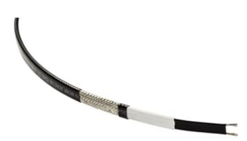
nVent RAYCHEM IceStop self-regulating trace heating cables provide roof and gutter de-icing, suitable for all standard materials of gutters and drainpipes. Power output is 36 W/m at 0  $^{\circ}$ C in ice water, 18 W/m at 0  $^{\circ}$ C in air.
