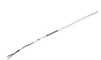
nVent RAYCHEM FMT constant wattage parallel trace heating cables provide freeze protection and process temperature maintenance, up to 150 °C. They can withstand routine steam purges and intermittent exposure to 200 °C, 230 V supply and FEP outer jacket. Approved for use in hazardous areas.
