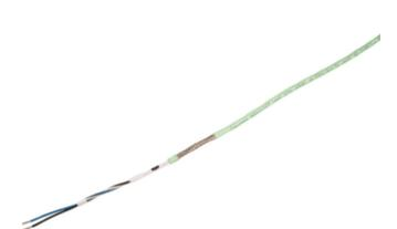
nVent RAYCHEM FHT constant wattage parallel trace heating cables provide freeze protection and process temperature maintenance, up to 230 °C. They can withstand routine steam purges and intermittent exposure to 260 °C, available in 230 and 400 V and approved for use in hazardous areas. The fluoropolymer outer jacket (-CT) provides high chemical resistance against aggressive organics and corrosives.
