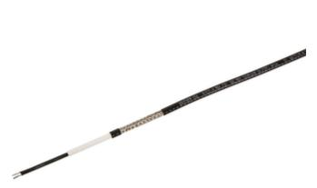
nVent RAYCHEM ETL self-regulating trace heating cables provide energy efficient pipe freeze protection. R-ETL-A/B are suitable for on- or in-pipe applications, R-ETL(-A/B)-CR for on-pipe only. Each are available in two power outputs (10 and 16 W/m at 5 °C), supported by a full range of heat shrinkable connections and accessories.
