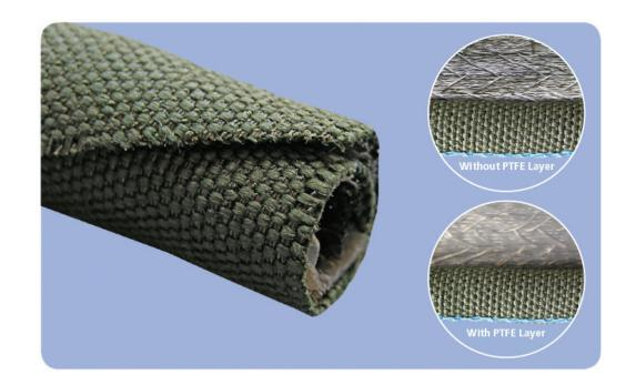
**ROUNDIT® 2000 NX EMI** is a self-wrapping sleeve designed for mechanical protection and EMI shielding of wire and cable bundles. The outer layer, which supplies the abrasion resistance, is manufactured from PPS monofilaments and Nomex\* with an oil and water repellent treatment. The inner layer is composed of nickel-plated copper (Cu/Ni), which provides EMI insulation. The outer layer construction with a 100% covering ratio provides excellent cut-through and abrasion resistance.
