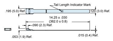
The 600-083 Extended Length Micro-Band is precision constructed of 300 Series SST/Passivate I.A.W. AMS 2700, and designed for use with the 600-061 Hand Banding Tool or the 600-068 Pneumatic Banding Tool. Double-wrapped bands will accommodate diameters up to approximately 1.88 inches (47.8). Bands may be ordered flat (600-083), or precoiled (600-083-1). Bands come bagged and tagged in quantities from 1 to 100.
