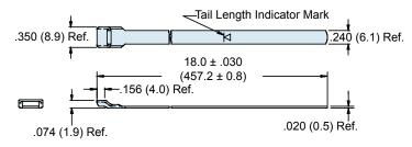
The 600-090 Extended Length Standard Band is precision constructed of 300 Series SST/Passivate I.A.W. AMS 2700, and designed for use with the 600-058 Hand Banding Tool or the 600-067 Pneumatic Banding Tool. Double-wrapped bands will accommodate diameters up to approximately 2.5 inches (63.5). Bands may be ordered flat (600-090), or precoiled (600-090-1). Bands come bagged and tagged in quantities from 1 to 100.
