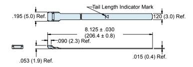
The 600-057 Micro Band is precision constructed of 300 Series SST/Passivate I.A.W. AMS 2700, and designed for use with the 600-061 Hand Banding Tool or the 600-068 Pneumatic Banding Tool. Double-wrapped bands will accommodate diameters up to approximately .88 inches (22.4). Bands may be ordered flat (600-057), or precoiled (600-057-1). Bands come bagged and tagged in quantities from 1 to 100.
