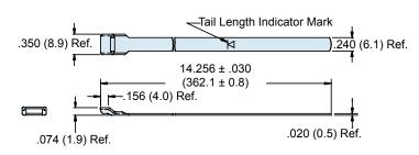
The 600-052 Standard Band is precision constructed of 300 Series SST/Passivate I.A.W. AMS 2700 and designed for use with the 600-058 Hand Banding Tool or the 600-067 Pneumatic Banding Tool. Double-wrapped bands will accommodate diameters up to approximately 1.8 inches (45.7). Bands may be ordered flat (600-052) or precoiled (600-052-1). Bands come bagged and tagged in quantities from 1 to 100.
