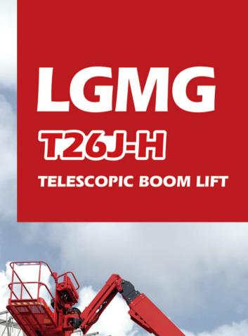
LGMG has a complete line of engine-driven, high-capacity telescopic boom aerial work platforms, with the maximum working height ranging from 21.8 to 29.8 meters (71'6"/97'9"). With a double capacity design of 450/300kg (992/661lbs), the machine can allow up to 3 people to work at the same time both indoors and outdoors, which greatly improves work efficiency.
